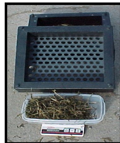
Weighing refusals and the Penn State Particle Separator
