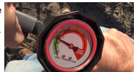
Soil penetrometer for detection of soil compaction.
